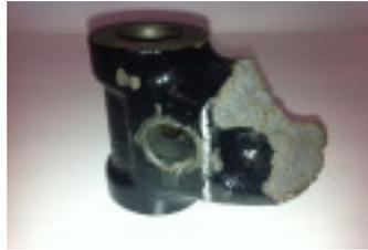
An investigation by the LVVTA, working closely with foundries and metallurgists, found a major manufacturing problem with the casting process used in the production of the batch that included the failed New Zealand axle.
